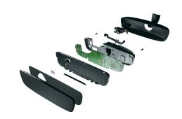
Magna's unique driver and occupant monitoring system combines camera, electronics and the interior mirror in one unit
